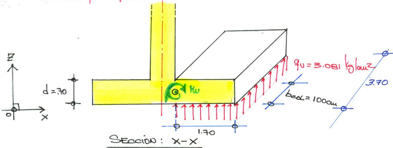
$$M_w = \frac{q_u L^2}{2} b_{\text{eff}} \Rightarrow M_w = \frac{3.081 (1.70)^2 (100)}{2} \Rightarrow M_w = 44.52 \text{ ton-m}$$
