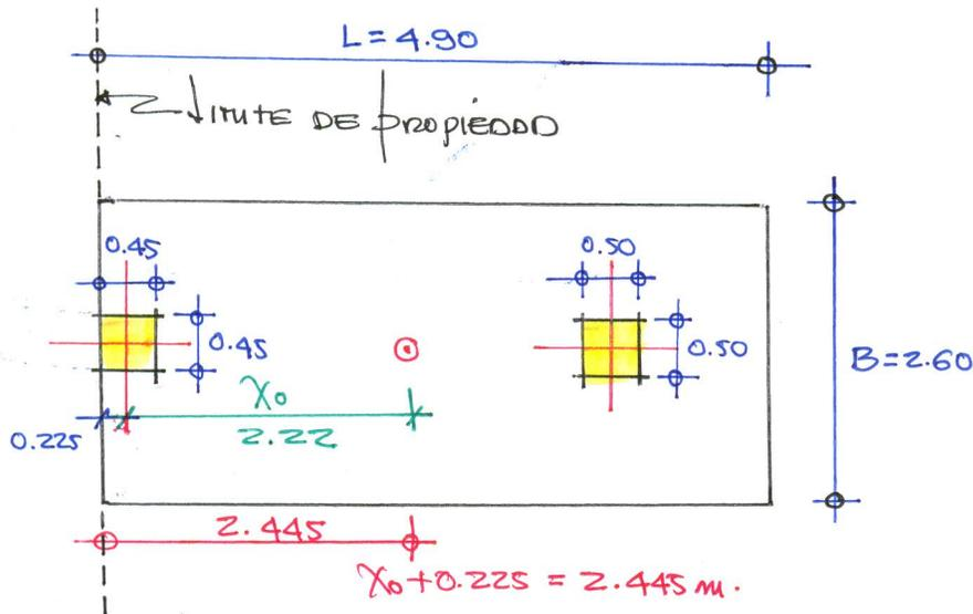
LONGITUD DE LA ZAPATA  $\downarrow = 2(2.445) \Rightarrow L = 4.89 \Rightarrow \underline{L = 4.90 \text{ m}}$
