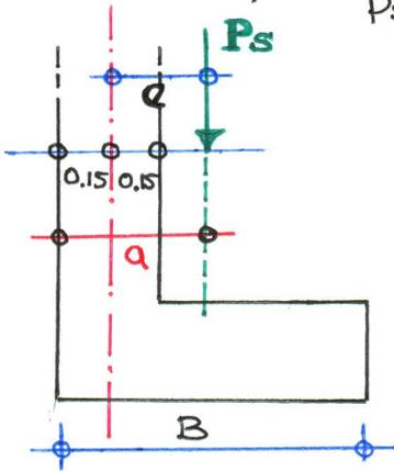
$$B_{\min} = 3e \Rightarrow B_{\min} = 0.681 \text{ m}$$
