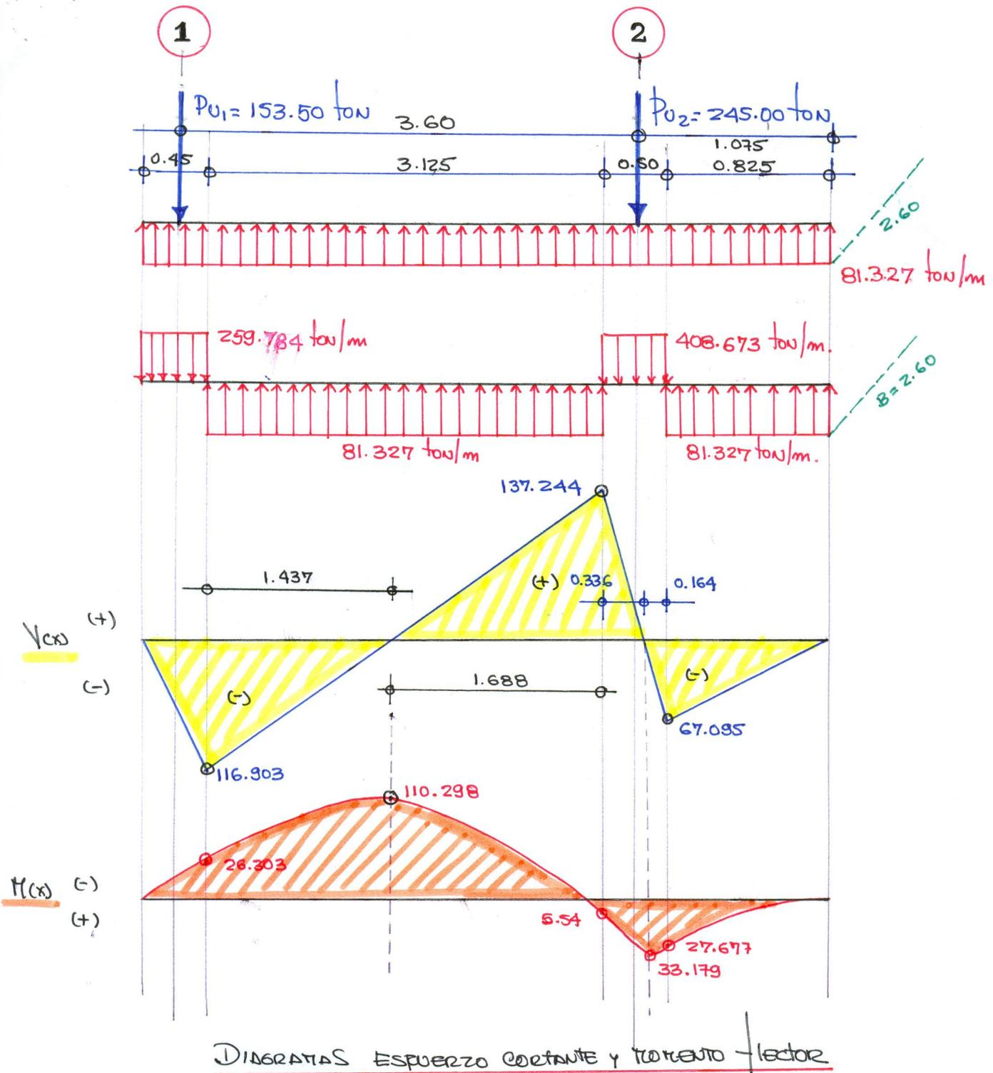
VERIFICACION CORTE FLEXION:  $B=2.60$ ,  $L=4.90$ ,  $A=12.74 \text{ m}^2$   $d=60 \text{ cm}$ .
