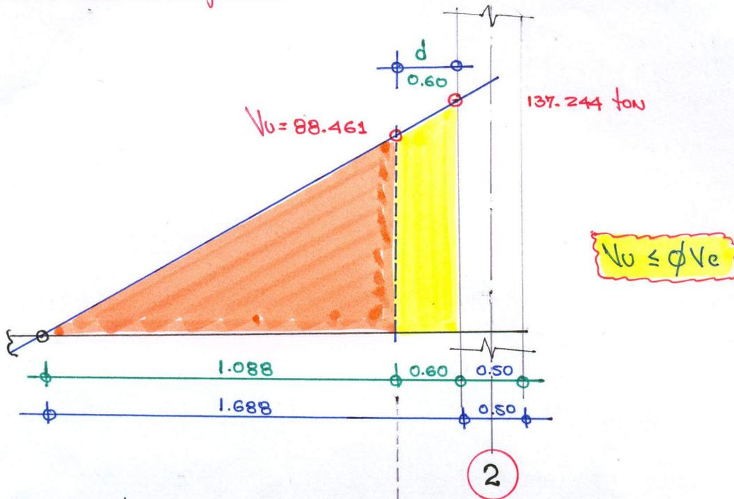
$V_u = 88.461 \text{ ton}$        $\phi V_c = \phi 0.53 \sqrt{f_c} B d = 0.85 \times 0.53 \sqrt{28} \times 260 \times 60 = 117.597 \text{ ton}$
